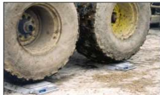
Figure 1: With portable scales, weigh each axle separately.
