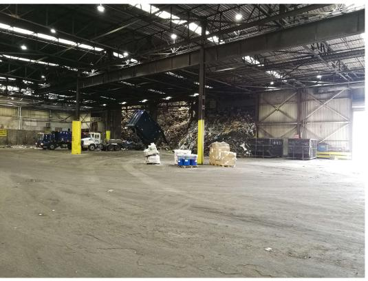
• Waste is unloaded onto the tipping floor throughout the day. It is managed by facility personnel to ensure that a good blend of material is deposited into the waste bunker for adequate mixing by the crane cab.
