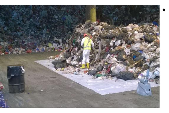
Depending on what material is identified and whether the truck is needed, a radiological consultant can be brought on site to separate and isolate the material triggering the radiation portal. Once segregated the material will be isolated in a drum until its levels drop down below site background.
